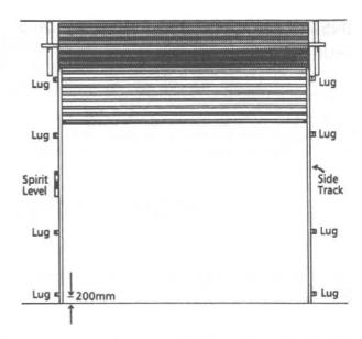
Slide the track on to the door curtain, allowing 4mm clearance. Hold the guide in position against the wall and mark the location of the top lug holding screw. USING A SPIRIT LEVEL TO ENSURE THAT THE SIDE TRACK IS ABSOLUTELY VERTICAL, fix the track in position by means of the adjustable lugs and 70mm coach screws ensuring that they are evenly spaced, with the bottom lug approximately 200mm from the floor.
